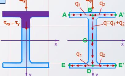
The shear flow at B into the web, the values of  $q$  corresponding to the two halves of the upper flange. After reaching a maximum value at C on the neutral axis and at D splits into equal parts corresponding to the two halves of lower flange.
