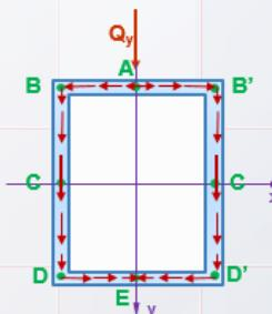
The shear flow  $q$  grows smoothly from zero at A to a maximum value at C and C' on the neutral axis, and then decreases back to zero at E is reached.
